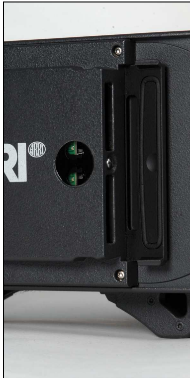
Figure 25: Camera left: SxS slots
